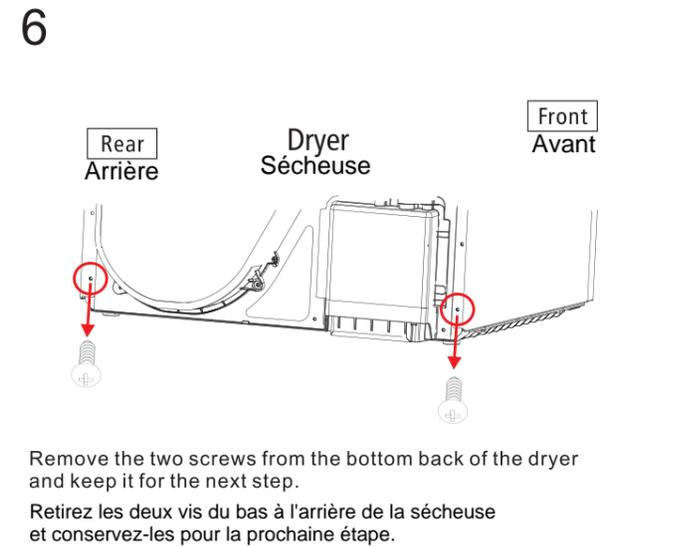
Remove the two screws from the bottom back of the dryer and keep it for the next step.
