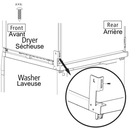
Secure part B to the dryer using Part A (x1).
